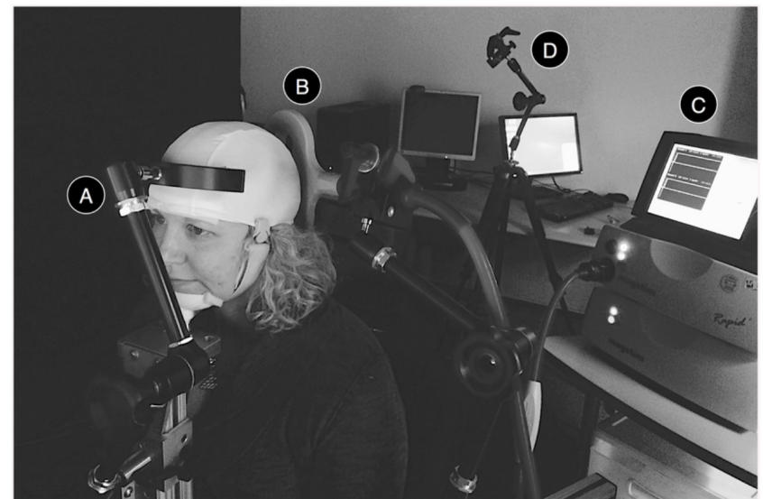
TMS Components of the BBI for the Inquirer. During the experiment, the inquirer sat in front of a computer screen on a BrainSight chair, with his or her head kept in place by a two-pronged head rest (A). A figure-of-8 TMS coil (B), connected to a MagStim Super Rapid2 stimulator (C) was positioned over the inquirer's occipital lobe to deliver visual stimulation in accordance with the respondent's answer. The head position and the coil position were carefully checked with the aid of a laser pointer (D).
